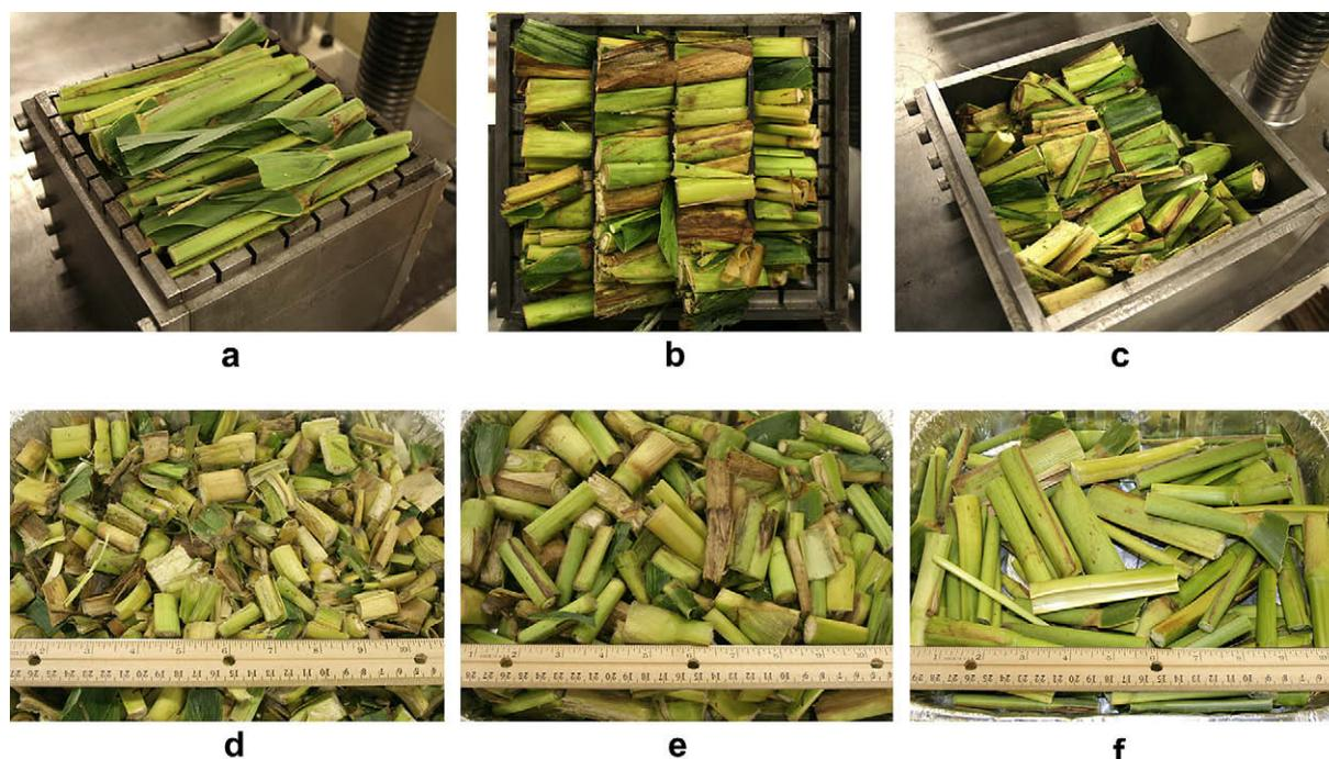
**Fig. 3 – Corn stalks size reduction at 50.8 mm knife grid spacing (a) loaded corn stalks above knife grid before cutting, (b) view from the underside of knife grid showing cut products caught in the knife grid, (c) cut products collected in the product block, (d) cut products from 25.4 mm knife grid spacing, (e) cut products from 50.8 mm knife grid spacing and (f) cut products from 101.6 mm knife grid spacing.**
